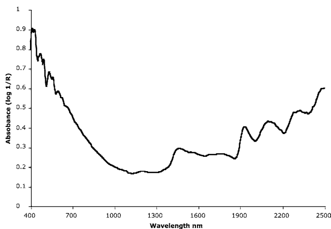
Figure 4. Typical spectrum showing diffusion reflectance ( R ) of dried, ground kava underground tissues over 400–2500 nm wavelengths.
